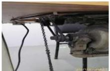
NC-7: In the sewing section, 4 sewing machine have no pulley covers.
